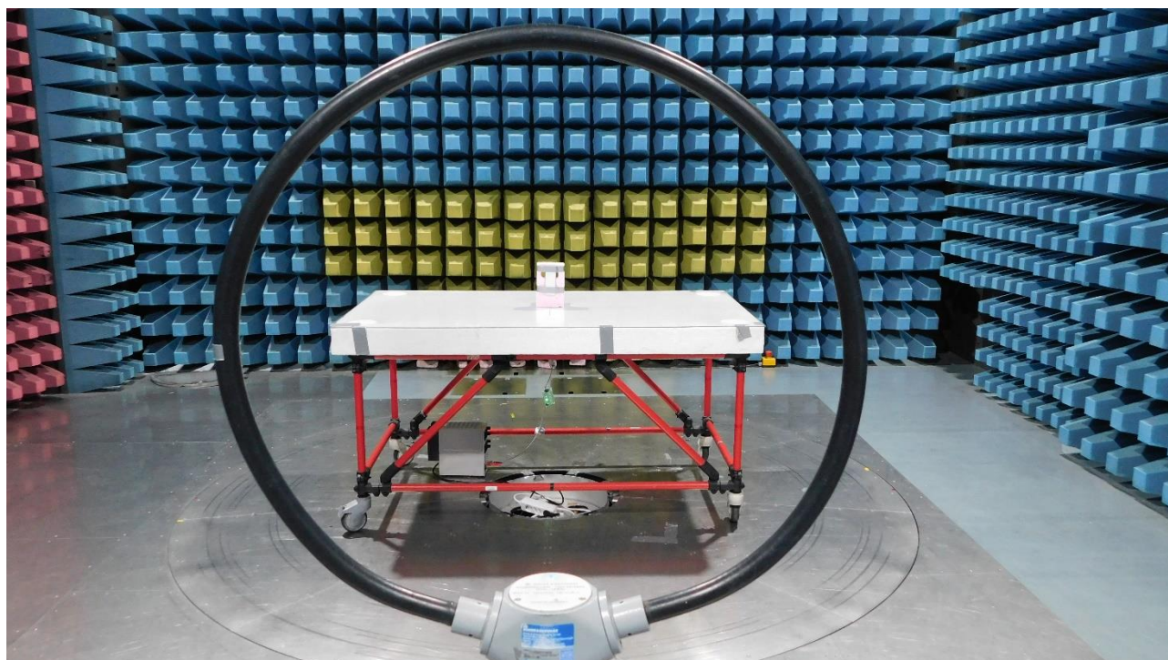
Picture 19: SAC, test setup radiated emission test 9 kHz - 30 MHz (rear view)
