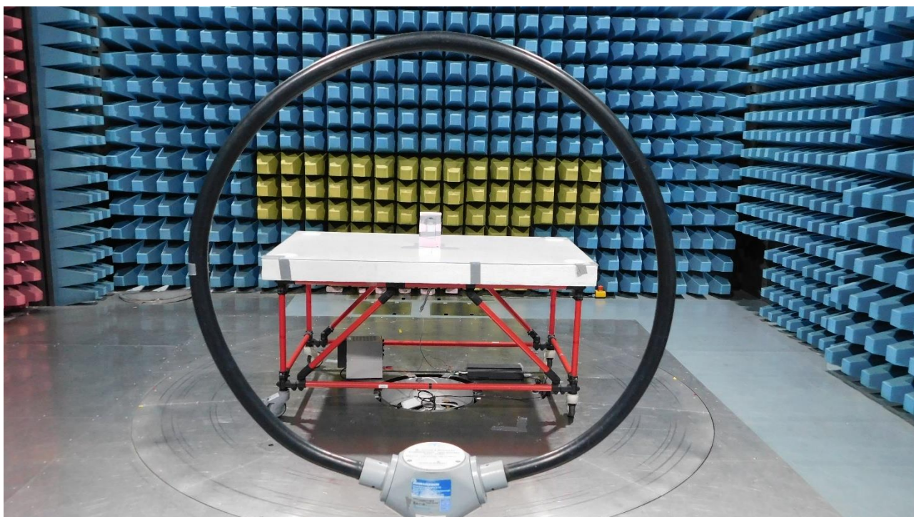
Picture 12: SAC, test setup radiated emission test 9 kHz - 30 MHz (rear view)
