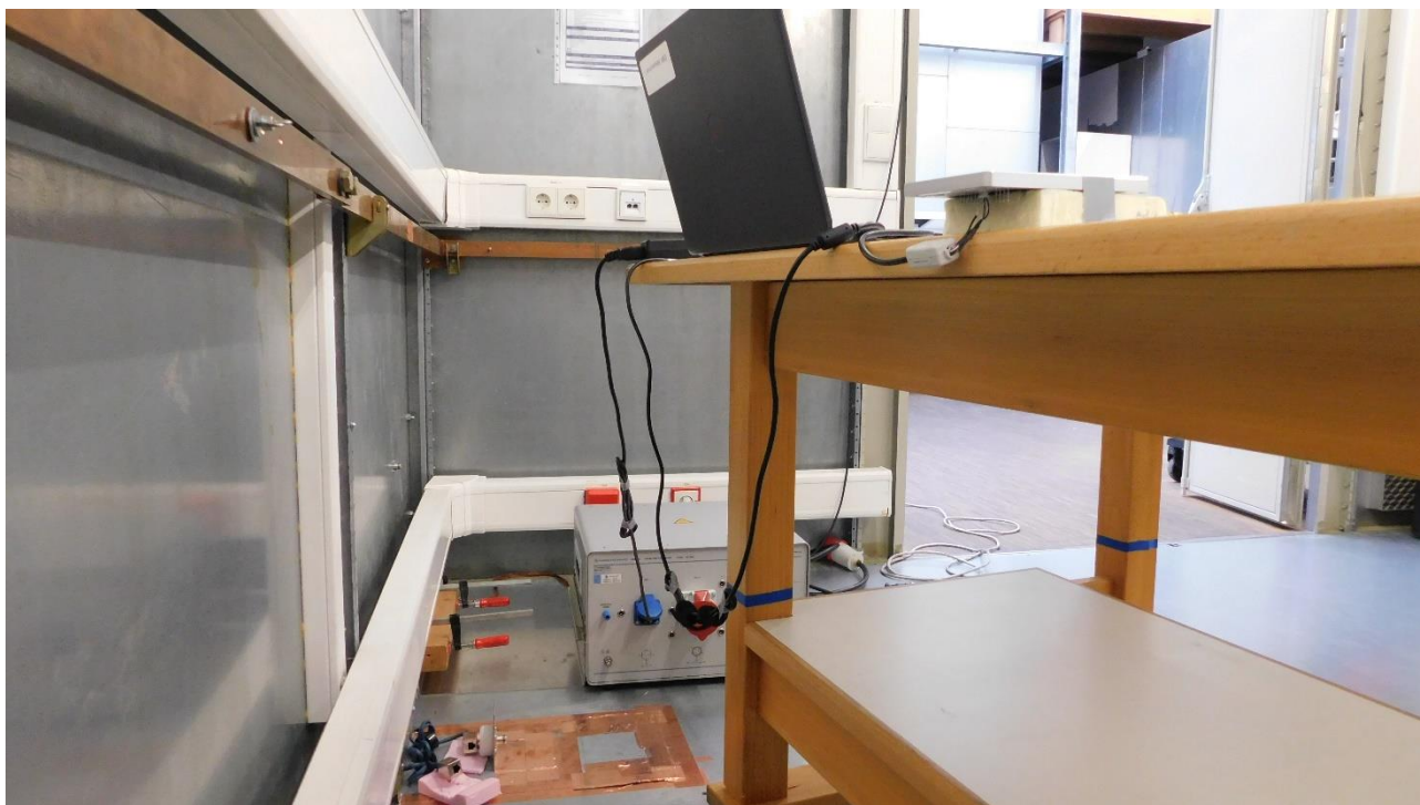
Picture 9: Test setup AC power line conducted emissions (rear view)
