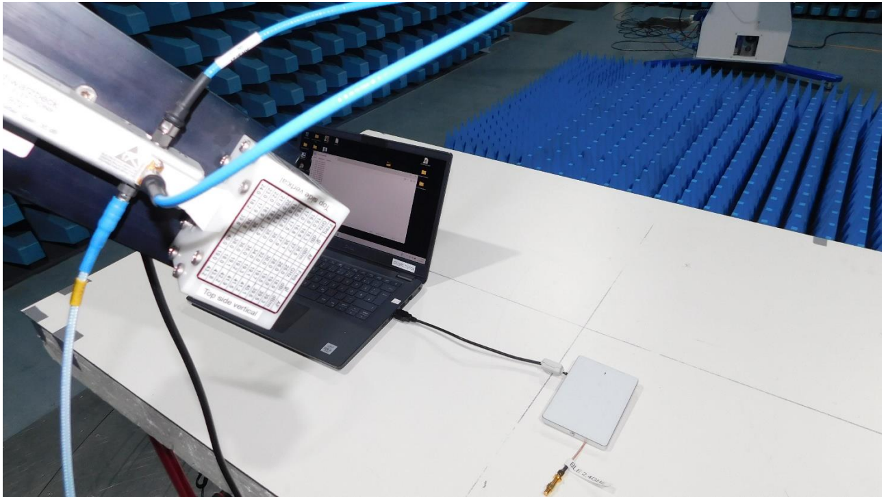
Picture 7: SAC, exploratory radiated emission test 17 GHz – 25 GHz (front view)
