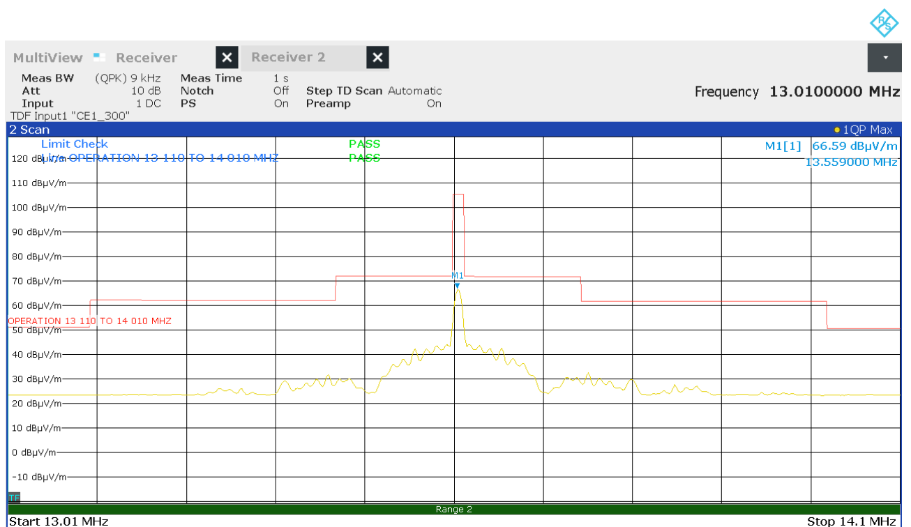
Figure 10: Chart of emission within the band 13.110 MHz to 14.010 MHz, EUT in position Z, without tag, antenna in line at 3 m distance
