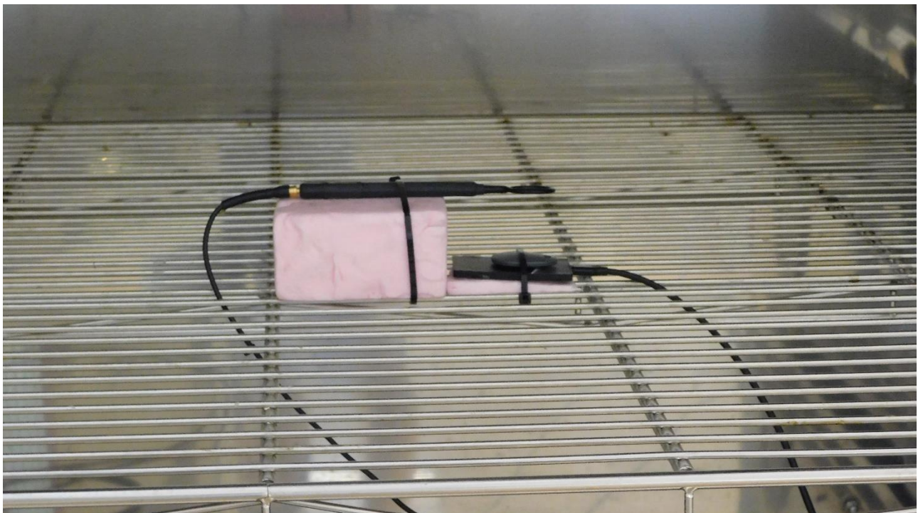
Picture 10: Test setup for carrier stability tests
