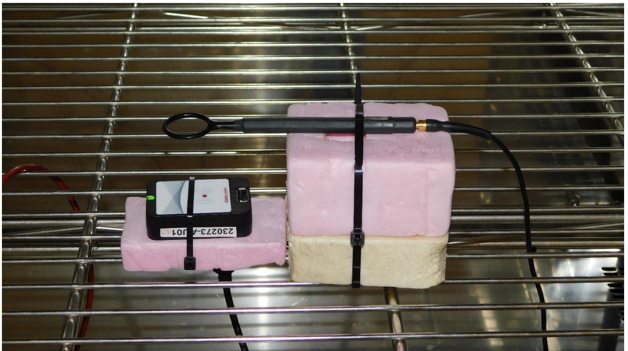
Picture 10: Test setup-Carrier frequency stability test
