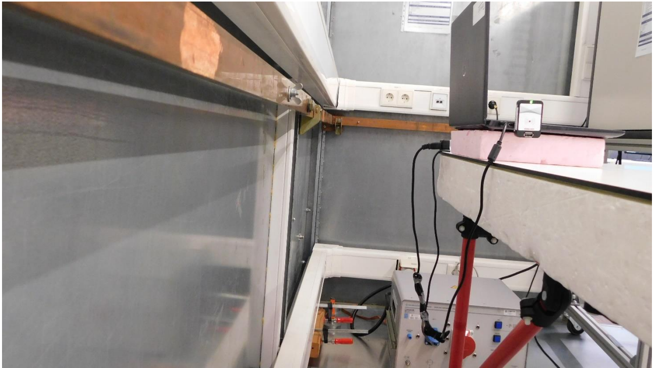
Picture 9: Test setup AC power line conducted emissions (rear view)
