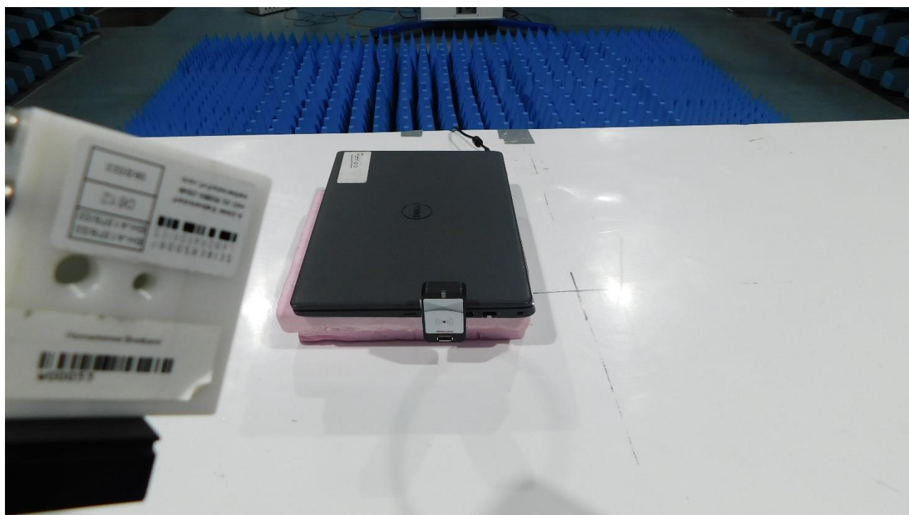
Picture 7: SAC, exploratory radiated emission test 17 GHz – 25 GHz (front view)
