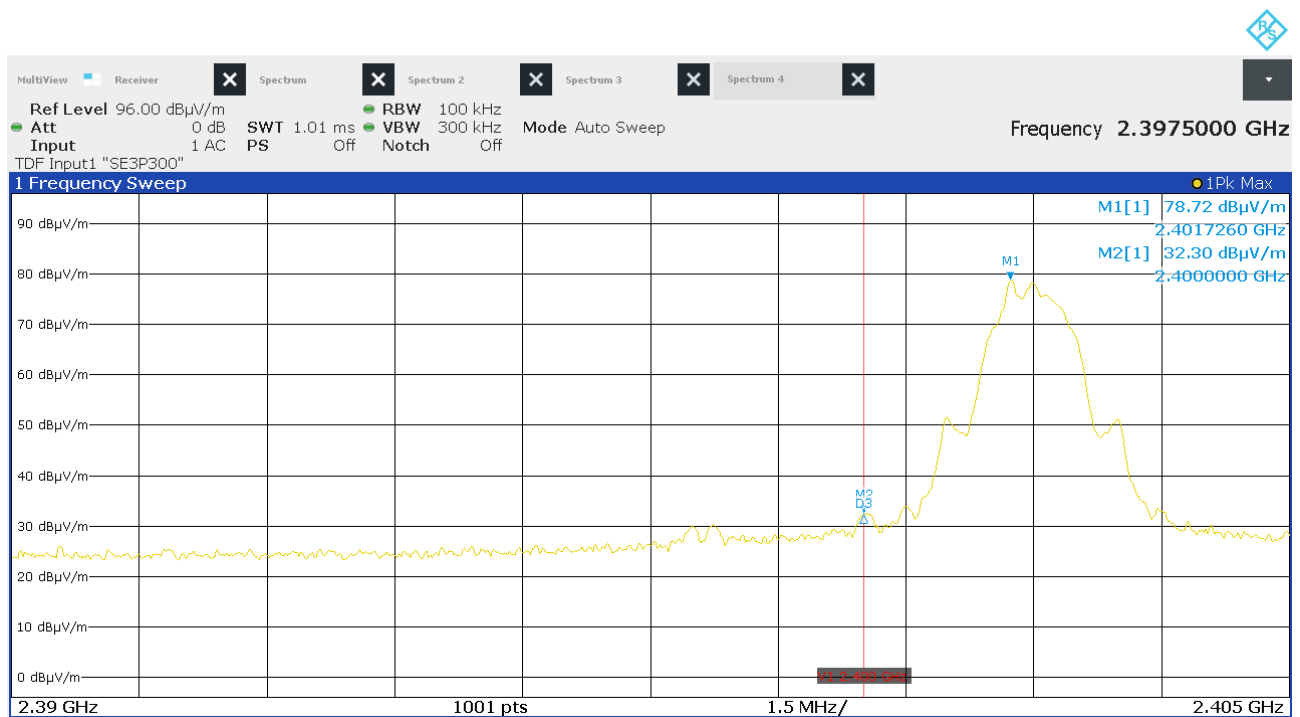
Figure 9: Chart of lower band edge measurement on lowest channel, EUT position X, antenna polarization horizontal
