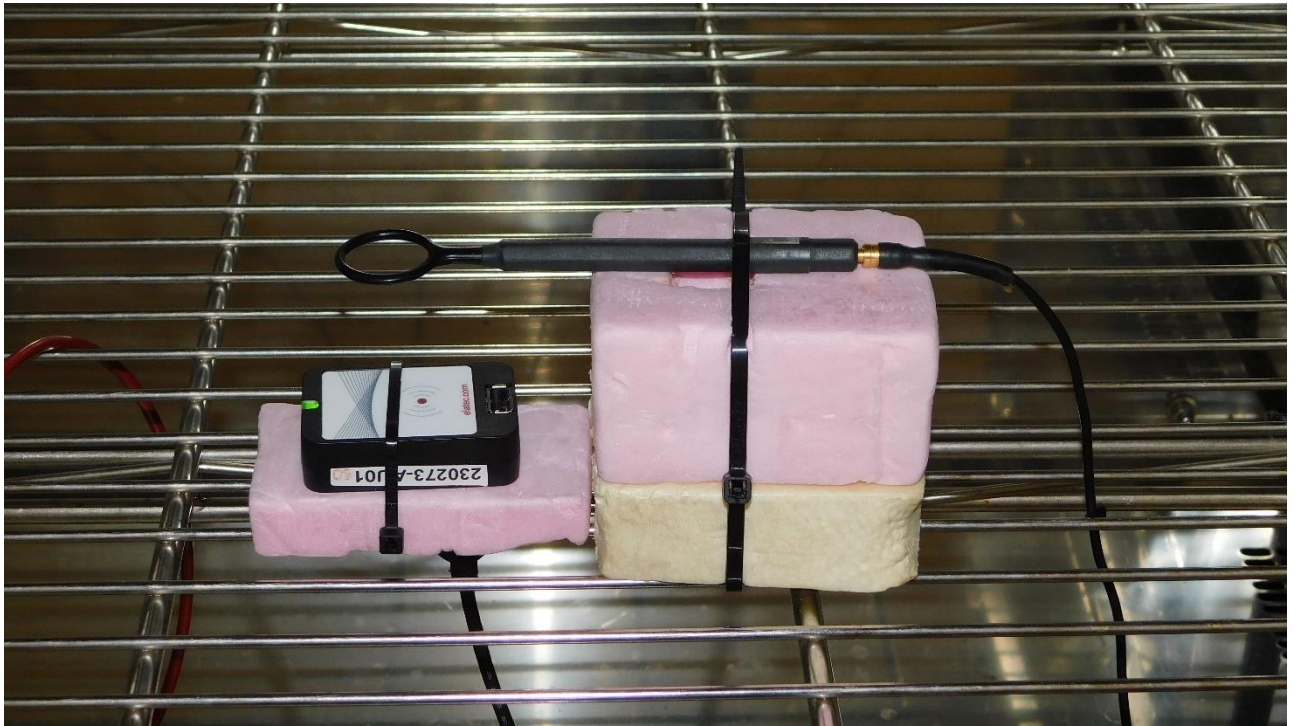
Picture 9: Test setup-Occupied bandwidth test
