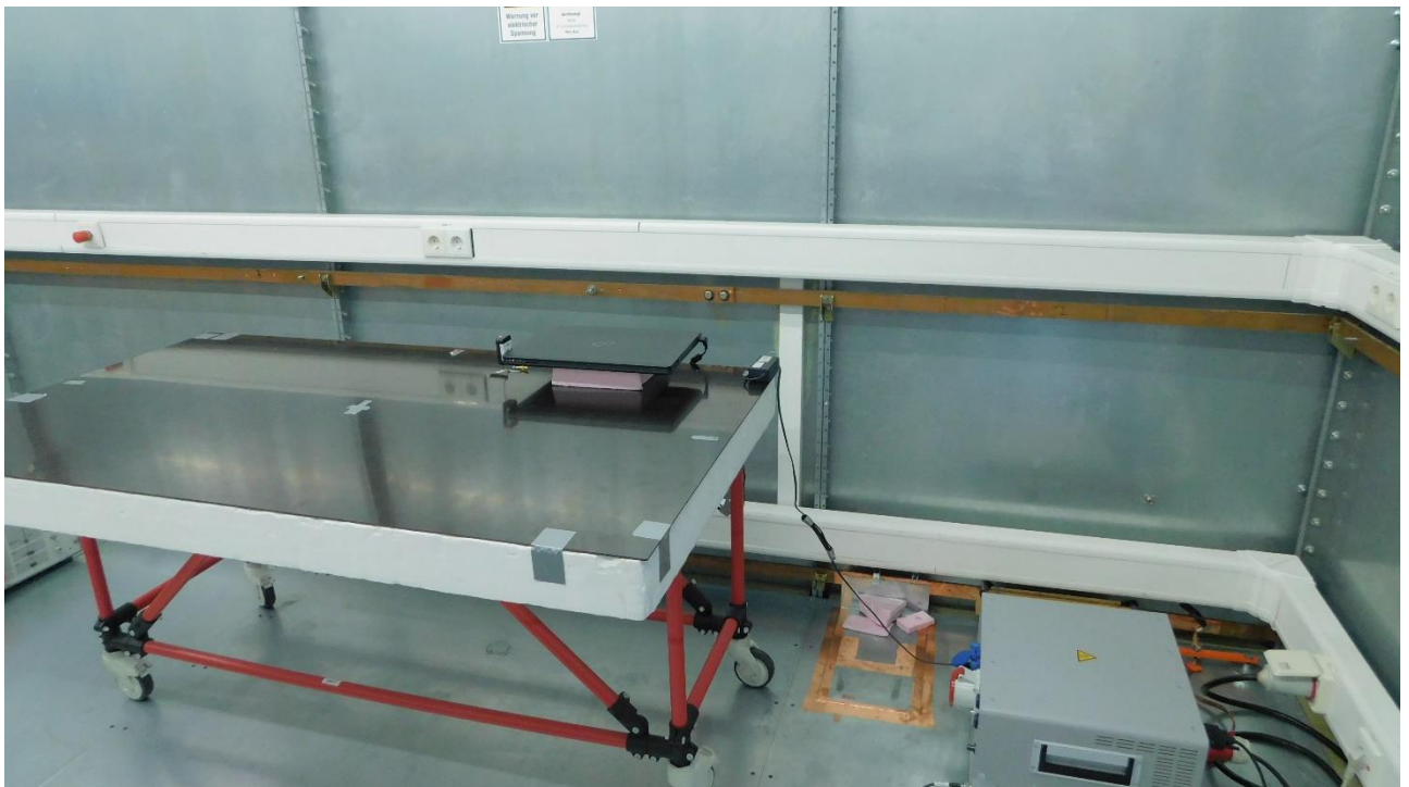
Picture 8: Test setup AC power line conducted emissions (front view)
