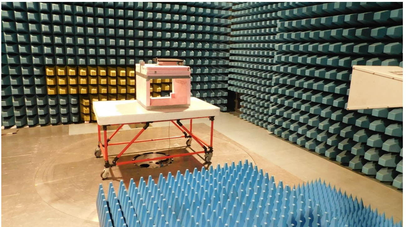
Picture 6: SAC, radiated emission test 1 GHz – 17 GHz (rear view)
