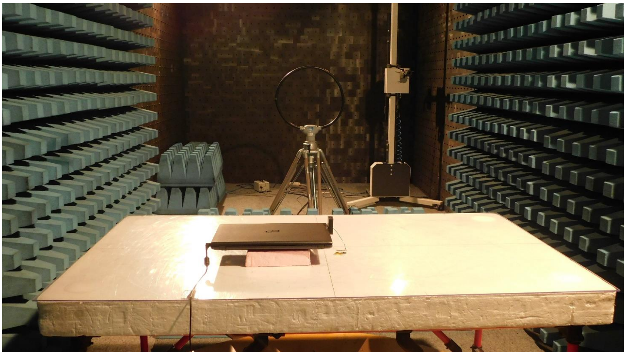
Picture 1: CDC, test setup radiated emission test 9 kHz - 30 MHz (front view)
