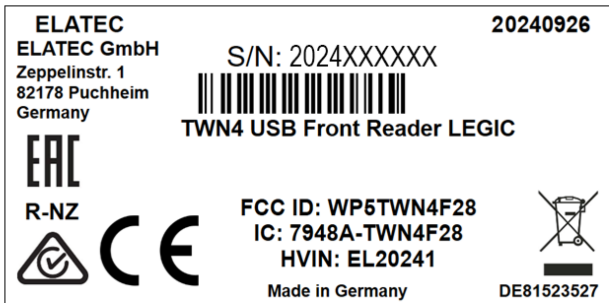
Picture 2: Name plate of EUT
