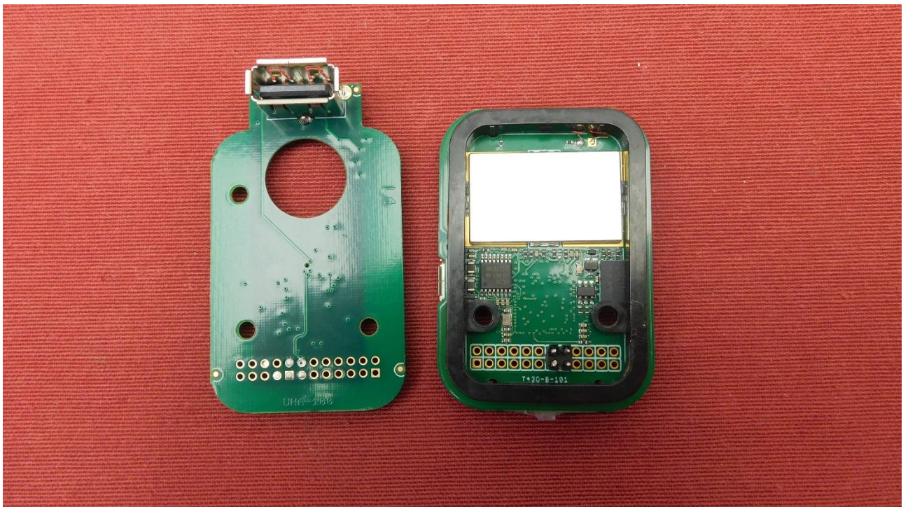
Picture 4: PCB 1 and 2 of EUT disassembled – bottom view
