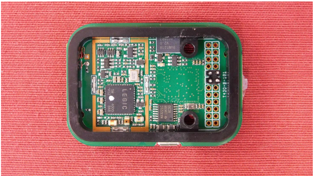
Picture 6: PCB 1 of EUT - bottom view without shielding
