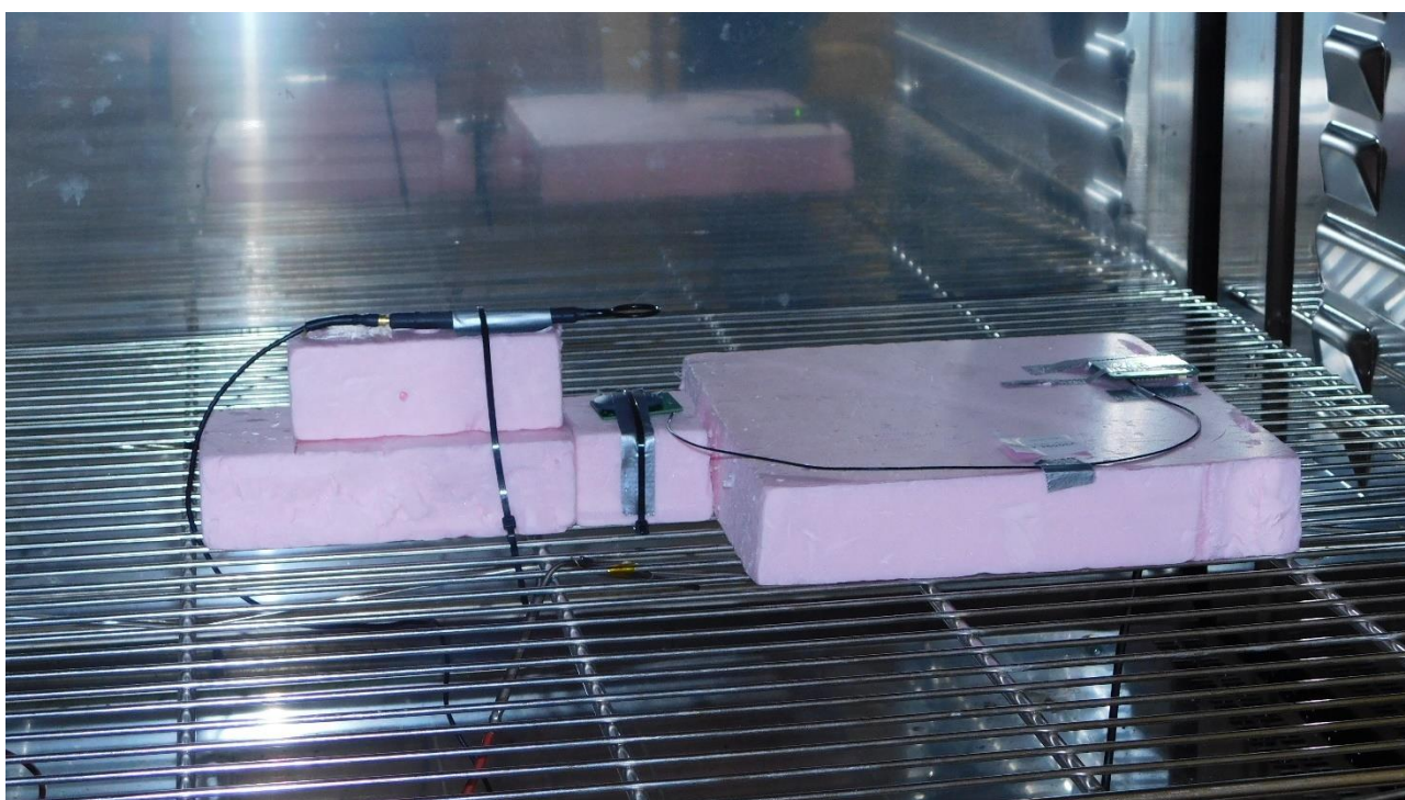
Picture 12: Carrier frequency stability test in climate chamber
