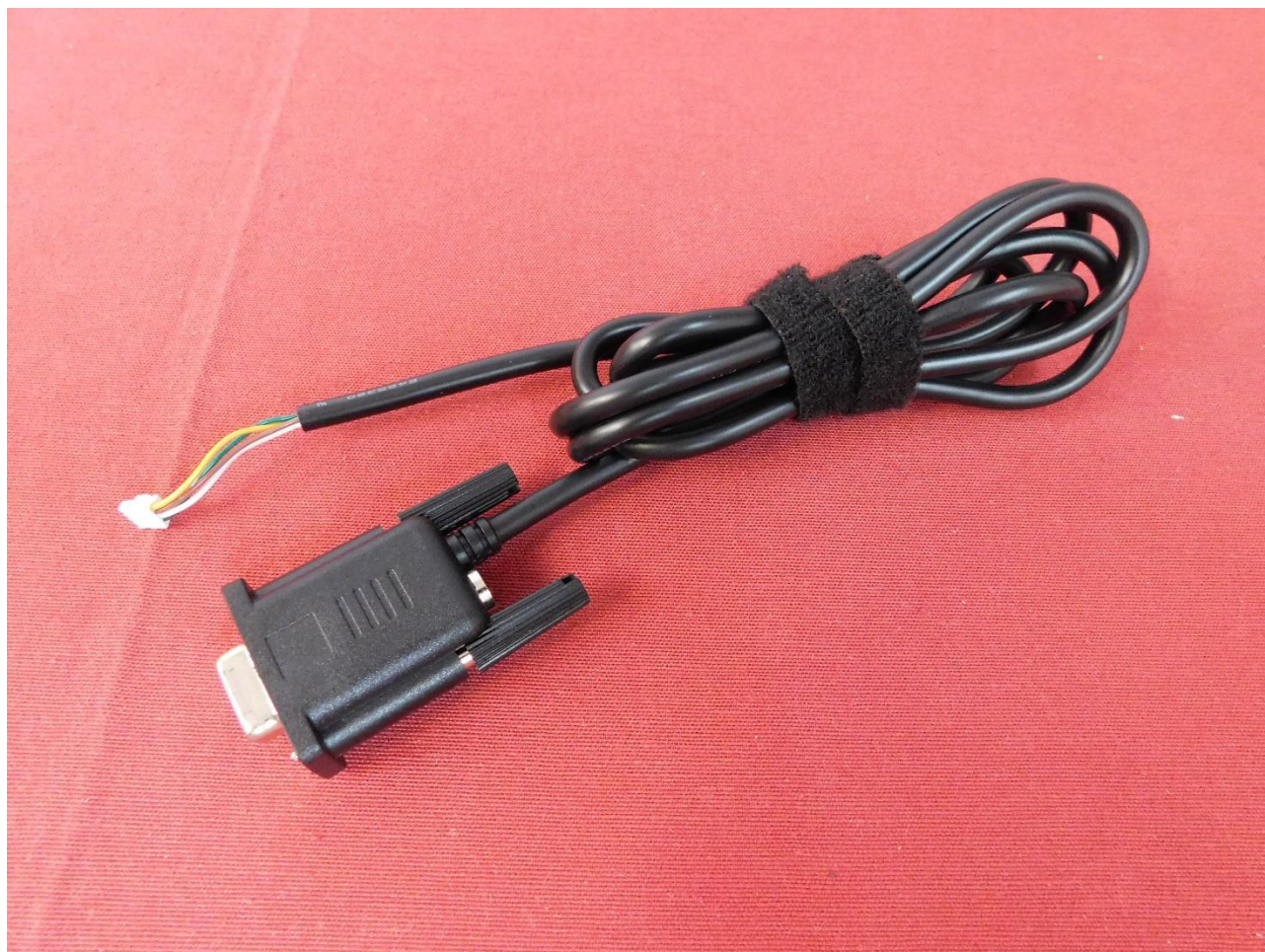
Picture 17: RS232 cable with DB9 connector
