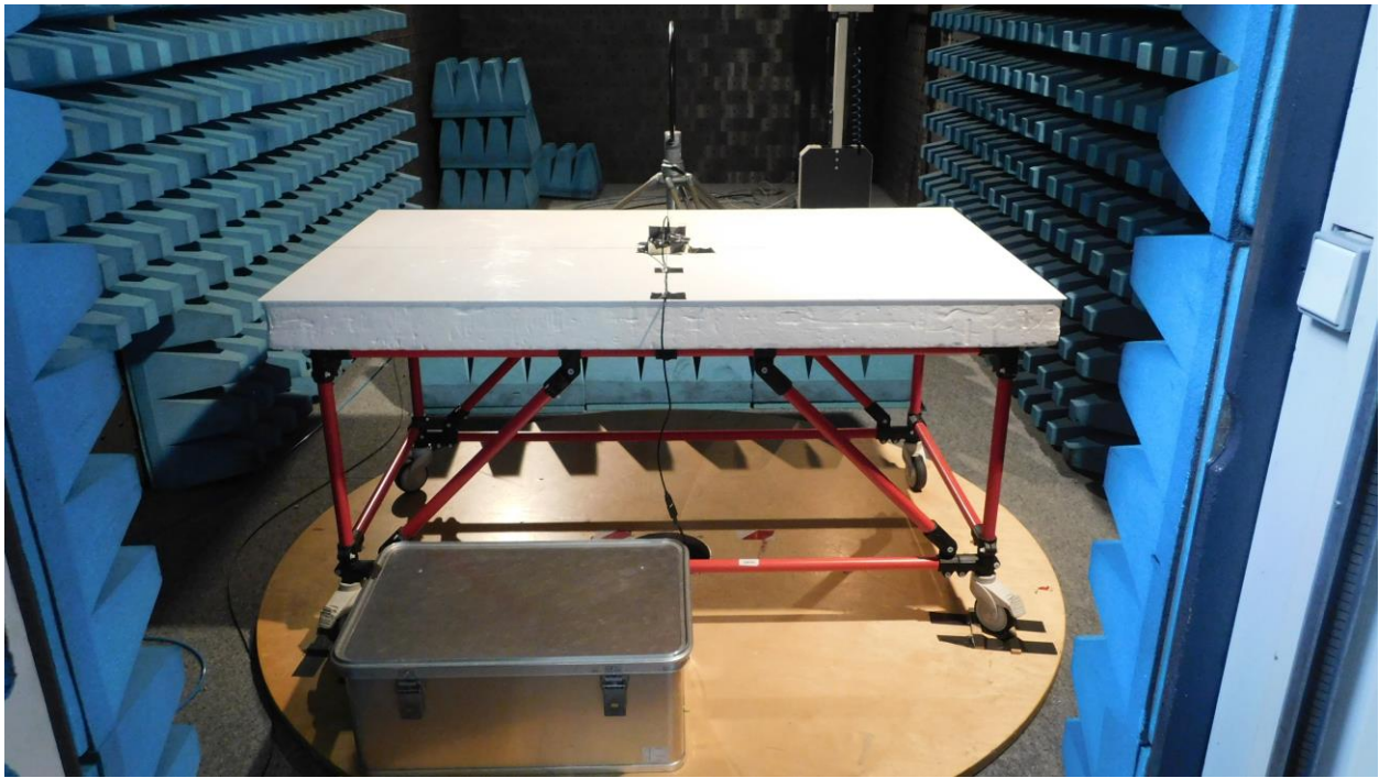
Picture 1: CDC, test setup radiated emission test 9 kHz -30 MHz (front view)
