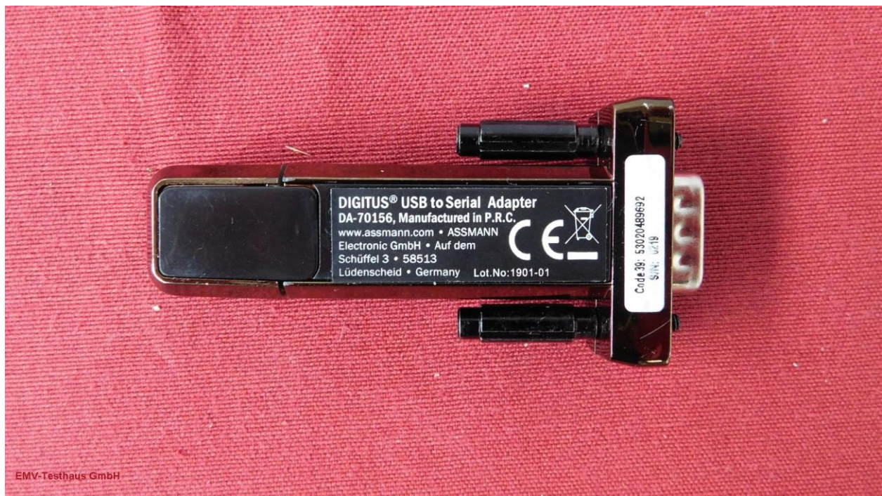
Picture 15: RS-232 – USB adaptor- bottom view
