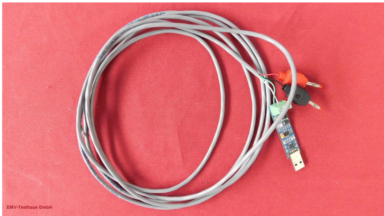
Picture 12: RS-485 adaptor + wiring
