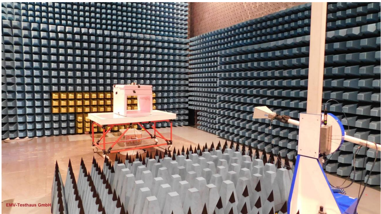
Picture 6: SAC, radiated emission test 1 GHz – 2 GHz (rear view)
