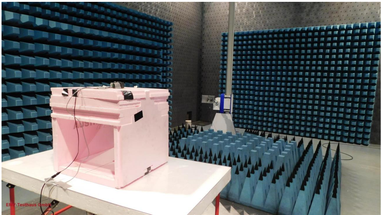
Picture 5: SAC, radiated emission test 1 GHz – 2 GHz (front view)
