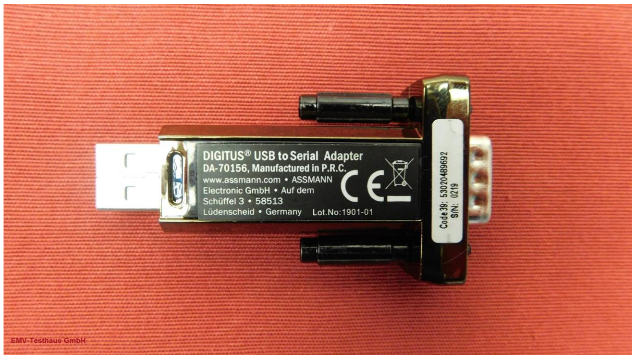
Picture 17: RS-232 to USB adapter – bottom side
