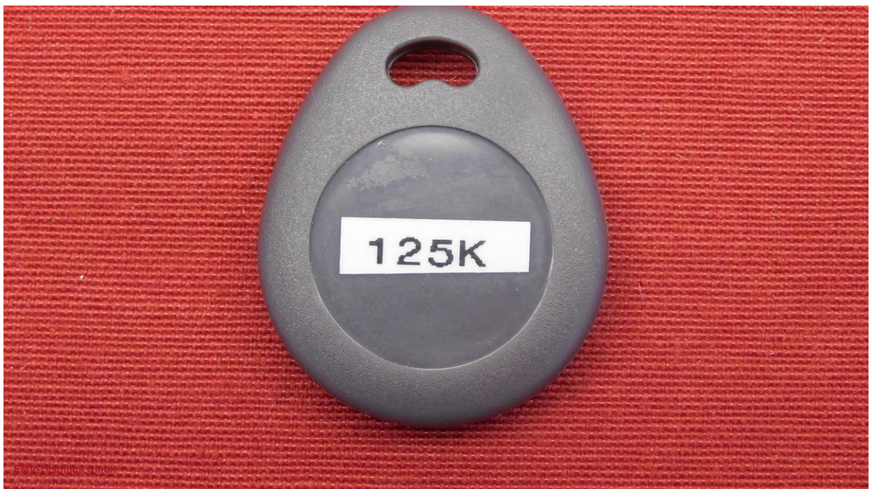
Picture 10: RFID tag 125 kHz top side
