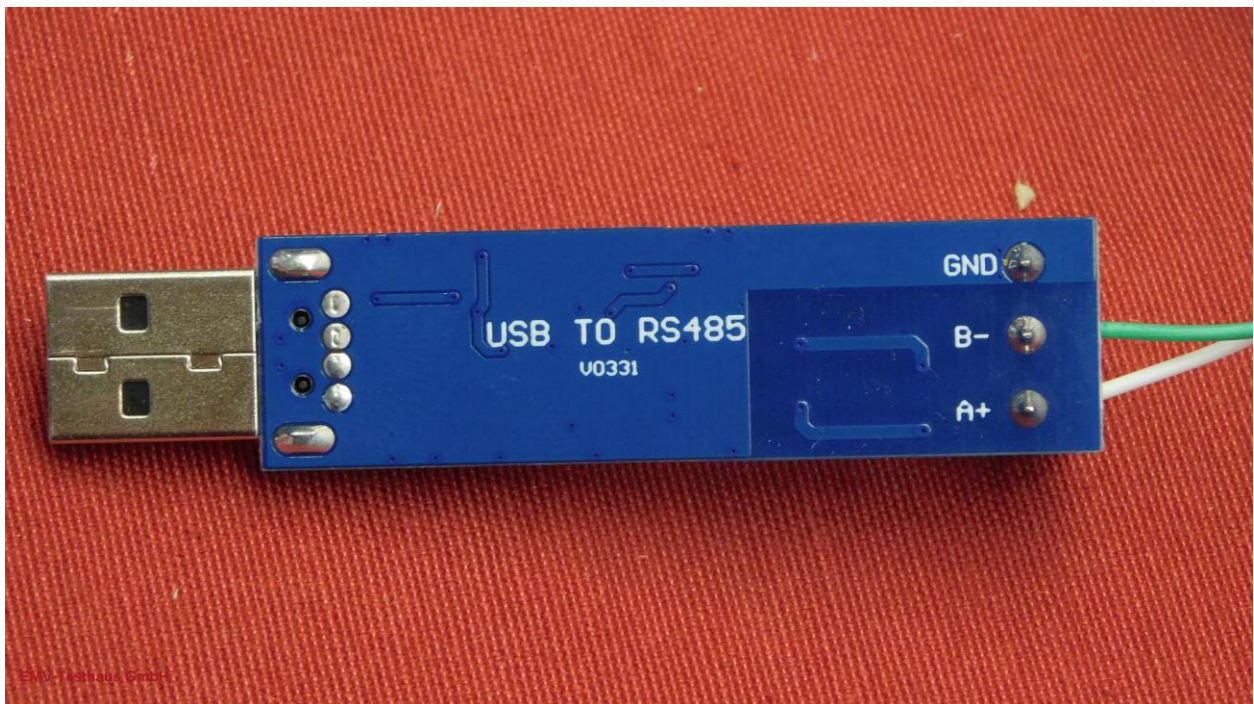
Picture 14: RS-485 to USB adapter – bottom side
