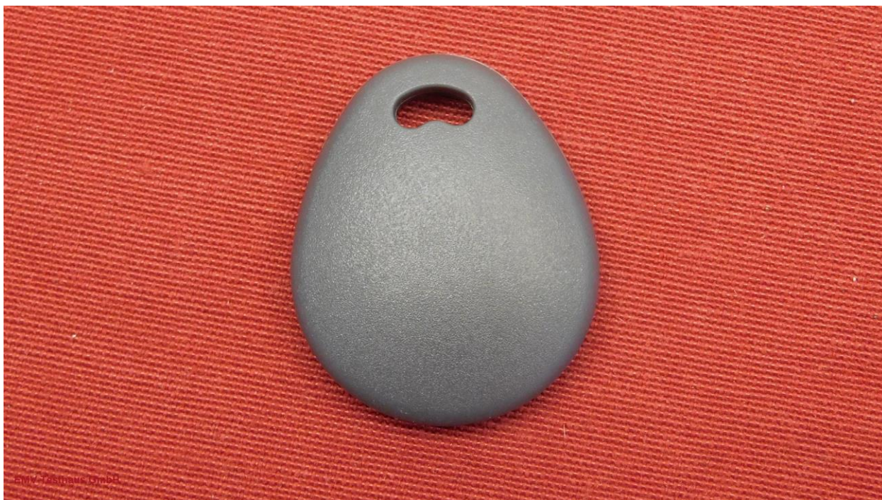
Picture 11: RFID tag 125 kHz bottom side
