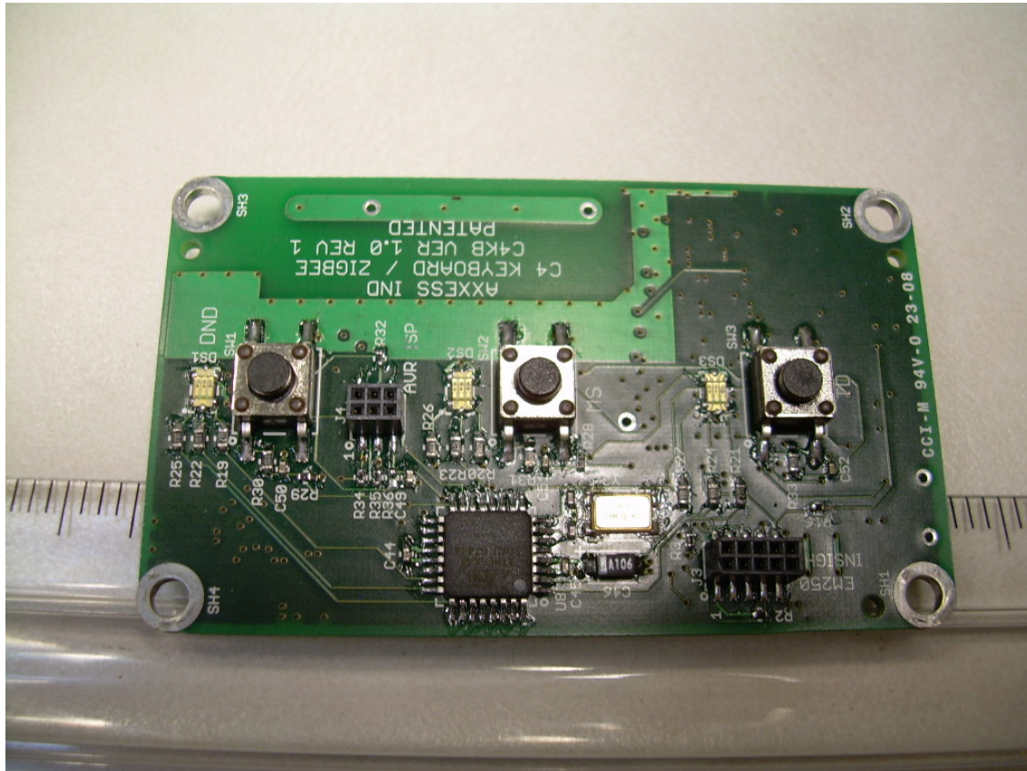
Front View of the RF PCB
