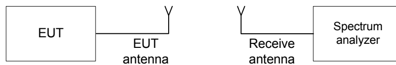
Figure 7.3.1 Occupied bandwidth test setup
