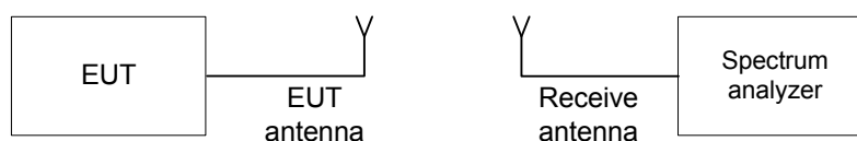
Figure 7.4.1 Band edge emission test setup
