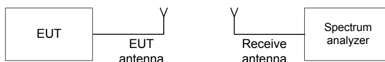
Figure 7.1.1 The 6 dB bandwidth test setup
