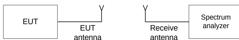
Figure 7.1.1 The 20 dB bandwidth test setup
