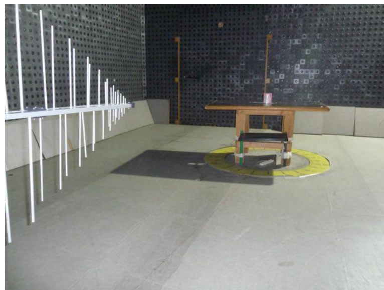
Photograph 8.1.1 Setup for radiated emission measurements
