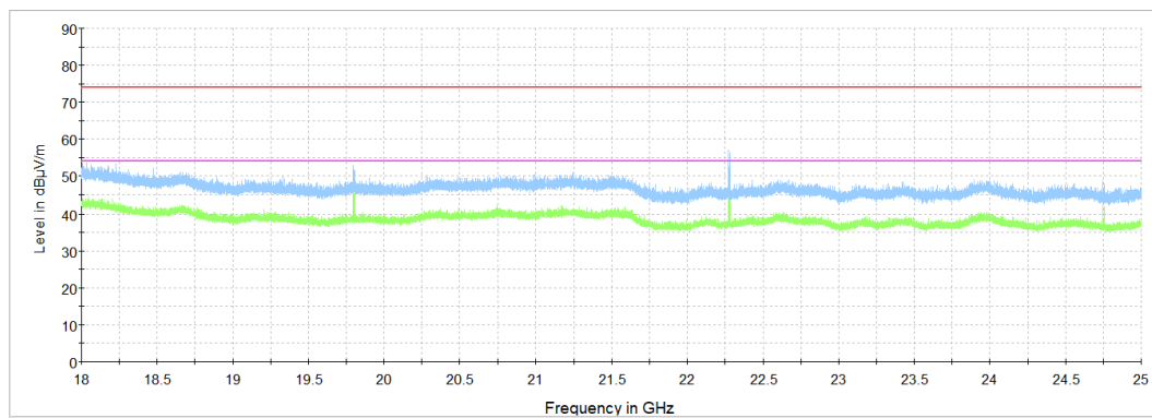
Plot 7.3.46 Radiated emission measurements from 18000 to 25000 MHz at the high carrier frequency Antenna 1
