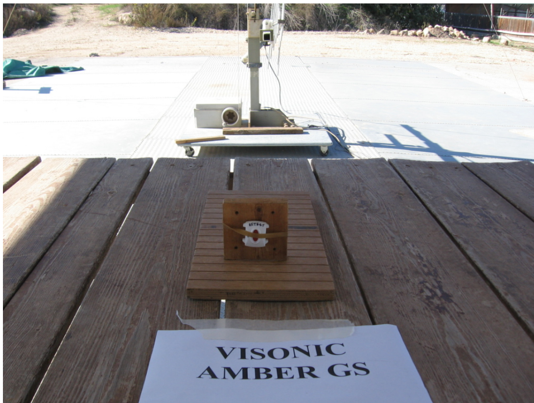
Figure 2 Radiated Emission Test Setup
