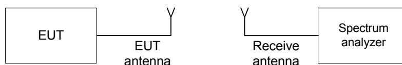
Figure 7.1.1 The 20 dB bandwidth test setup
