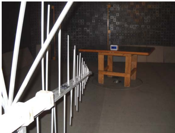
Photograph 8.1.1 Setup for preliminary radiated emission measurements
