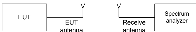
Figure 7.2.1 Carrier frequency separation test setup
