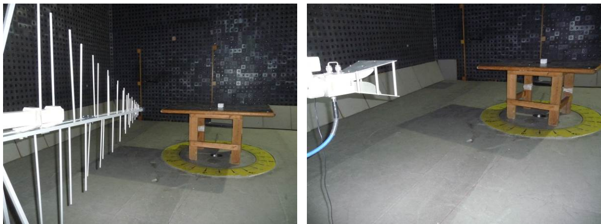
Photograph 7.7.1 Setup for radiated emission measurements
