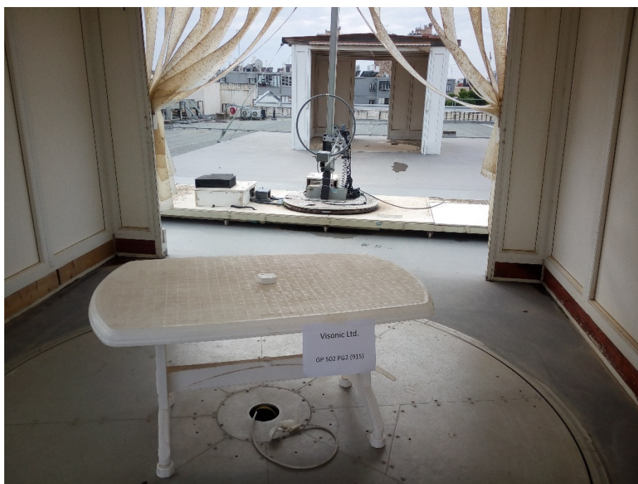
Figure 1. Radiated Emission Test – Ceiling Mounted
