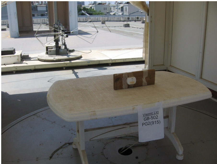
Figure 6. Radiated Emission Test – Wall Mounted
