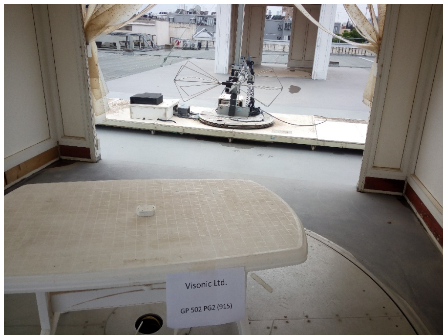
Figure 2. Radiated Emission Test – Ceiling Mounted
