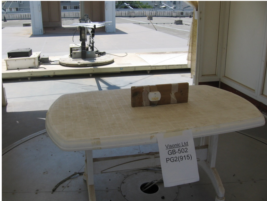
Figure 5. Radiated Emission Test – Wall Mounted
