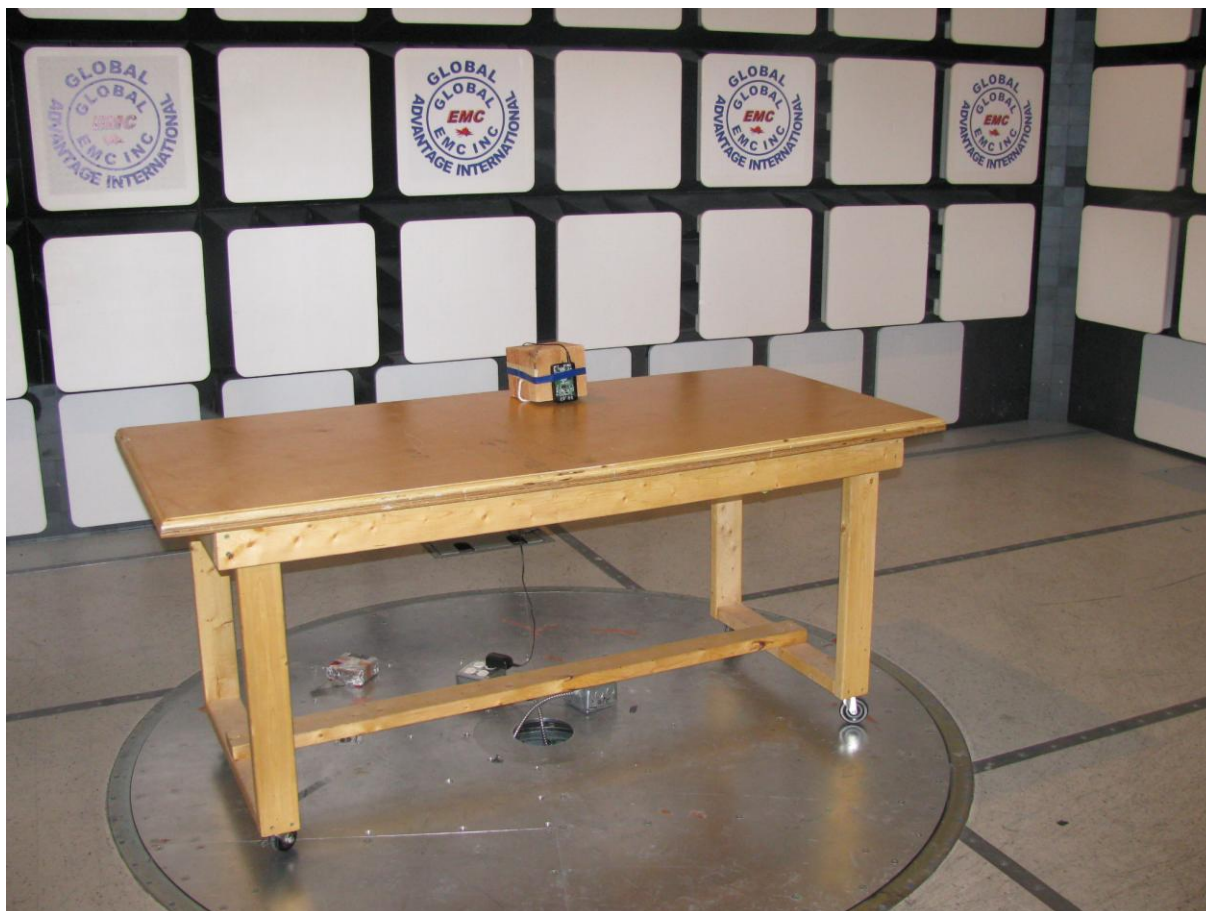
Figure 1 – Radiated emission setup
