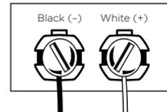
Loosen the terminals on your garage door opener but leave the wall control wires in place
