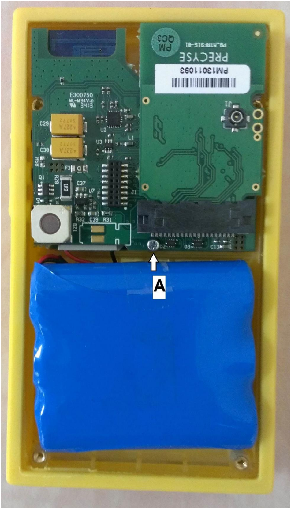
Photograph 8: ALL PCBs inside enclosure SA91/004135 (SA91/004035 with white enclosure)
