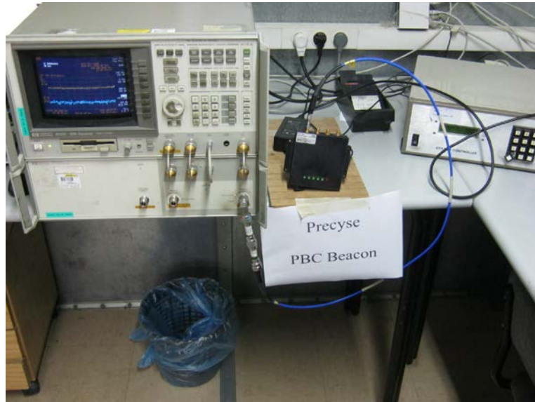
Figure 2. Conducted Emission From Antenna Ports Tests
