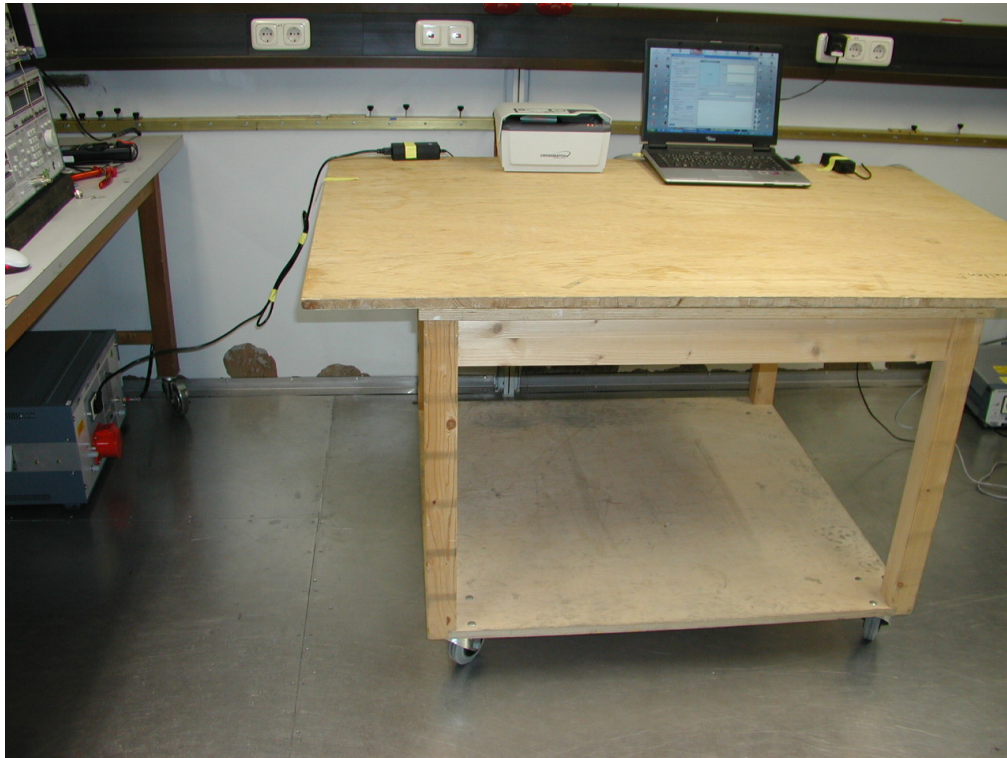
Figure 1 Arrangement for the measurement of conducted emissions
