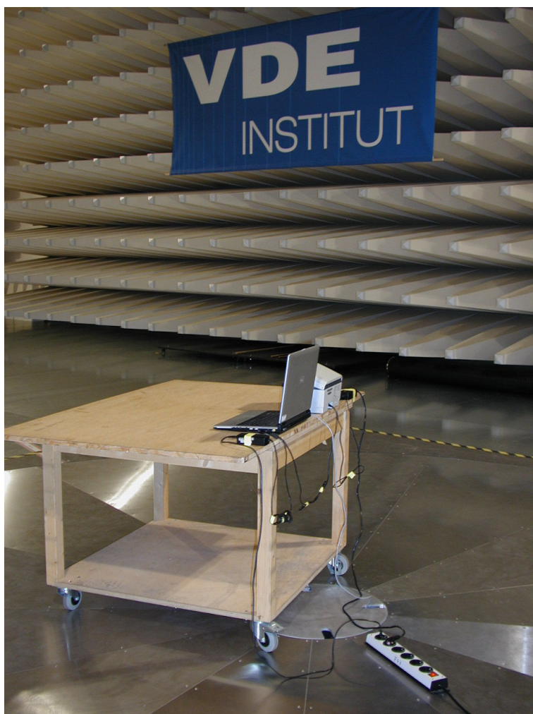
Figure 7 Arrangement for the measurement of radiated emissions
