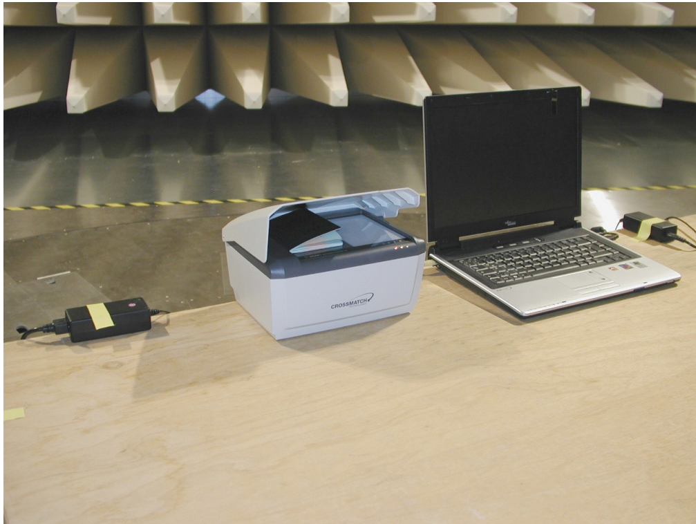
Figure 5 Arrangement for the measurement of radiated emissions
