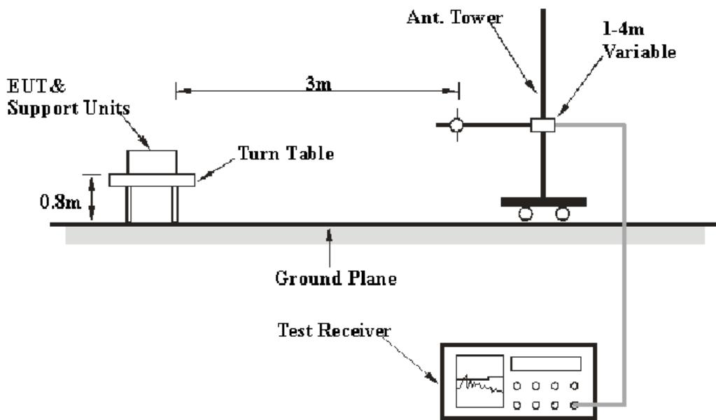
The radiated emission and out of band emission tests were performed in the 3 meters test site, using the setup accordance with the ANSI C63.4-2009. The specification used was the FCC 15.209 and FCC 15.249 limits.
