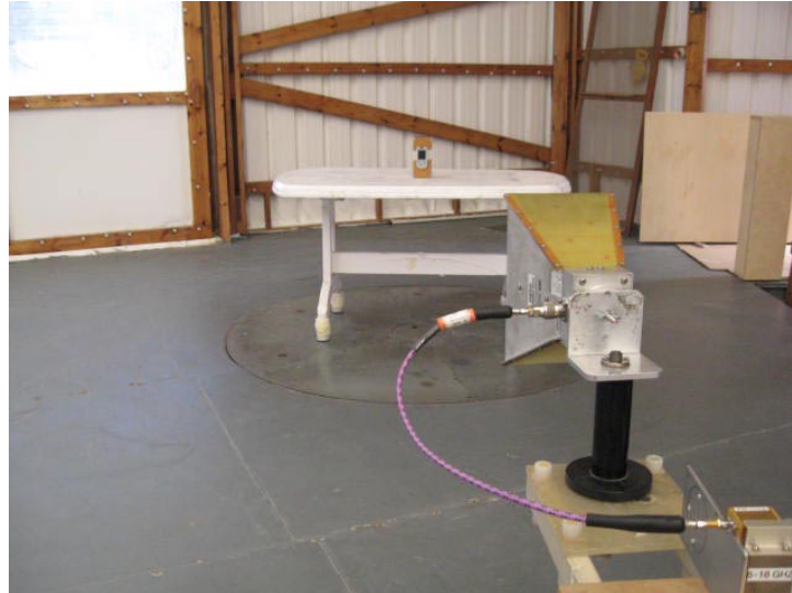
Photograph No.4 Setup for spurious emission measurements at OATS in 1 to18 GHz range
