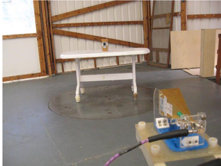
Photograph No.5 Setup for spurious emission measurements at OATS in 18 to 26.5 GHz range
