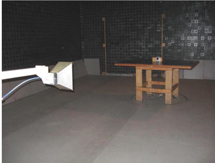
Photograph No.3 Setup for fundamental and spurious emission measurements in the anechoic chamber in 1 to18 GHz range, EUT in vertical position (X-axis)
