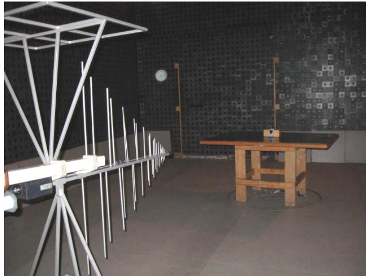
Photograph No.2 Setup for spurious emission measurements in the anechoic chamber from 30 MHz to 1 GHz, EUT in vertical position (X-axis)
