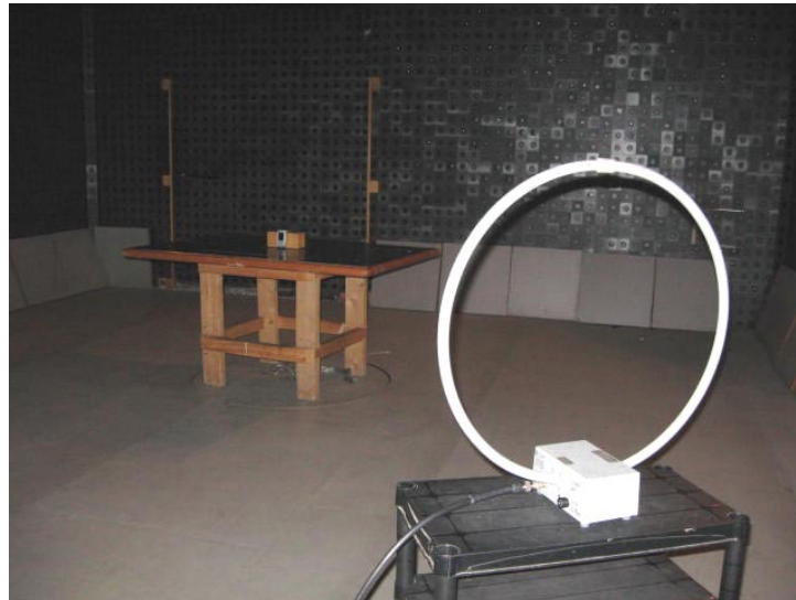
Photograph No.1 Setup for spurious emission field strength measurements in the anechoic chamber from 9 kHz to 30 MHz, EUT in vertical position (X-axis)
