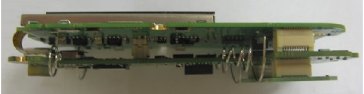
Photograph No.2 Remote Control unit internal side view
