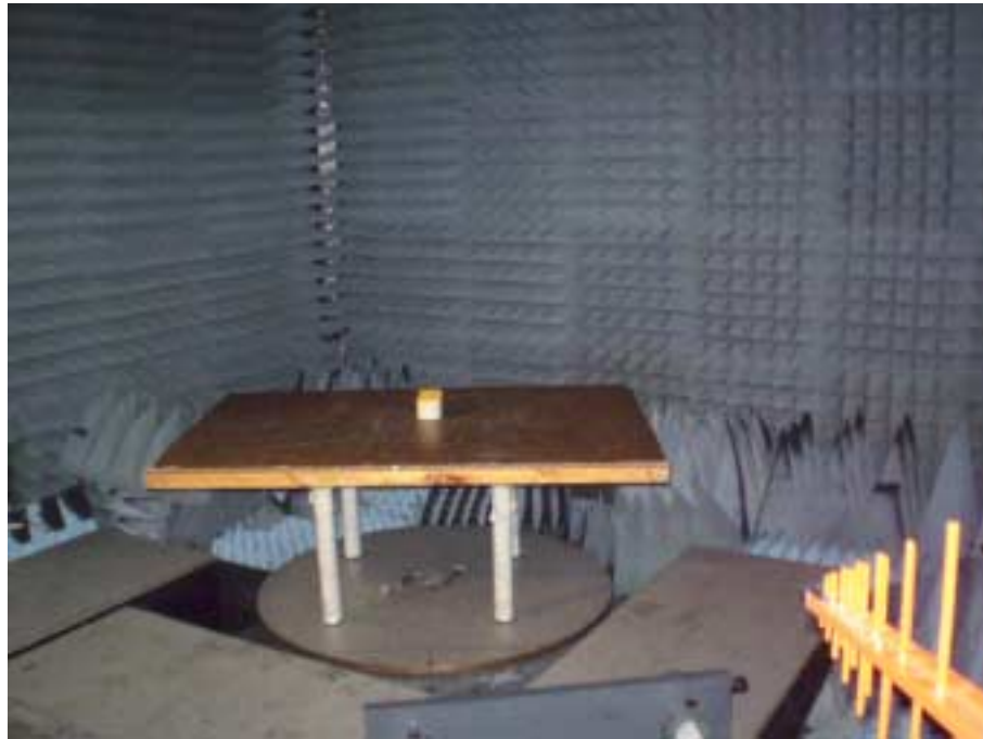
Photograph No.3 Setup for spurious emission field strength measurements in the anechoic chamber in 30 MHz-1000 MHz
