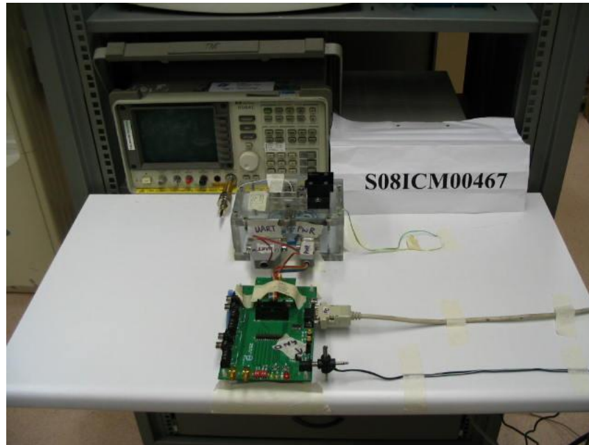
Average Frequency Dwell Time Test Setup
