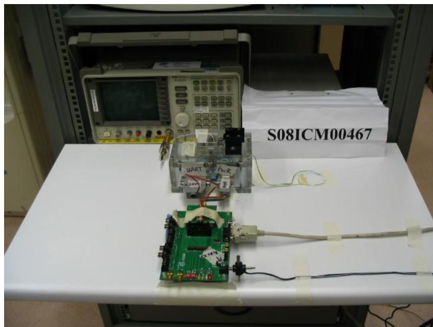
RF Conducted Spurious Emissions Test Setup
