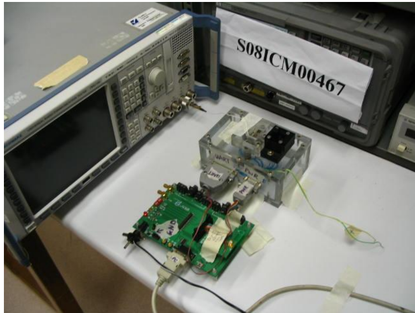
Maximum Peak Power Test Setup RF CONDUCTED SPURIOUS EMISSIONS TEST
