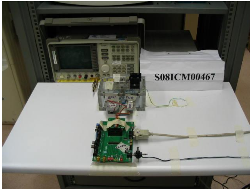
Carrier Frequency Separation Test Setup
