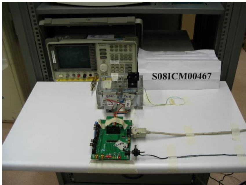
Spectrum Bandwidth (20dB Bandwidth Measurement) Test Setup
