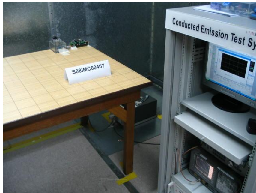
Conducted Emissions Test Setup (Front View)
