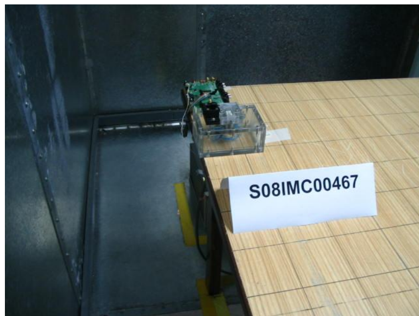
Conducted Emissions Test Setup (Rear View)
