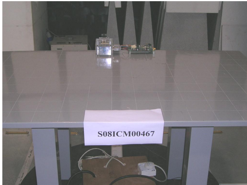
Radiated Emissions Test Setup (Front View)
