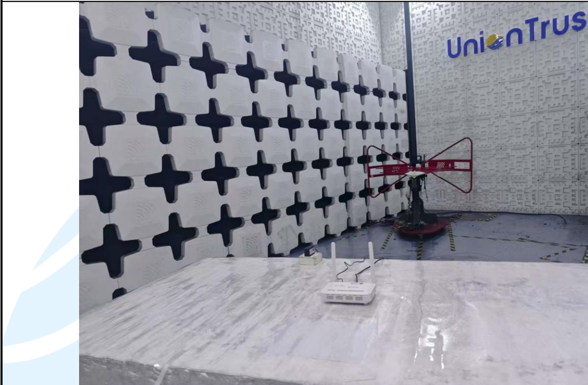
Radiated emission Test Setup (30 MHz~1 GHz)
