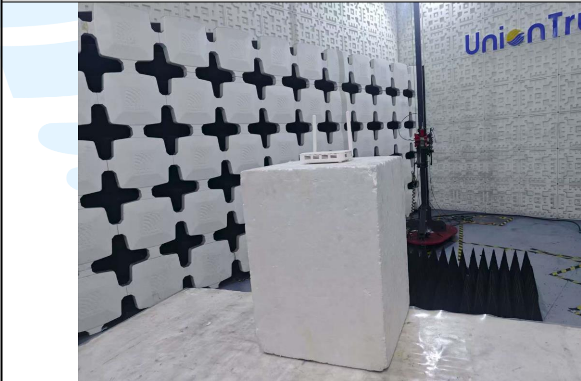
Radiated emission Test Setup (Above 1 GHz)
