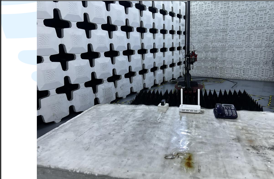
Radiated emission Test Setup-2 (Above 1 GHz)
