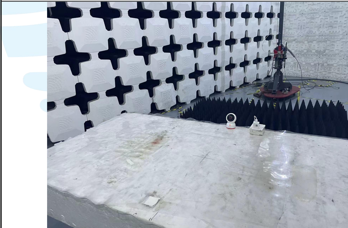
Radiated emission Test Setup-2 (Above 1 GHz)
