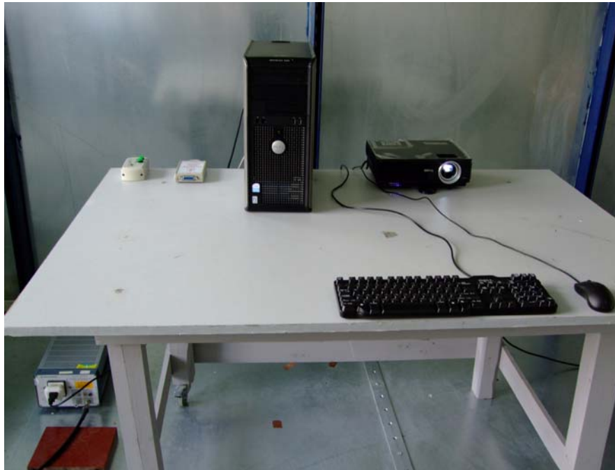
Conducted Emission Test Set-up - Front View
