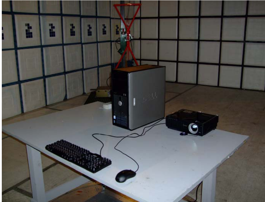
Radiated Emission Test Set-Up – Front View
