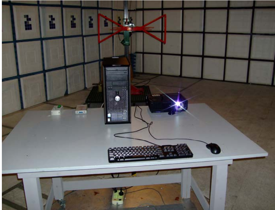
Radiated Emission Test Set-Up – Front View
