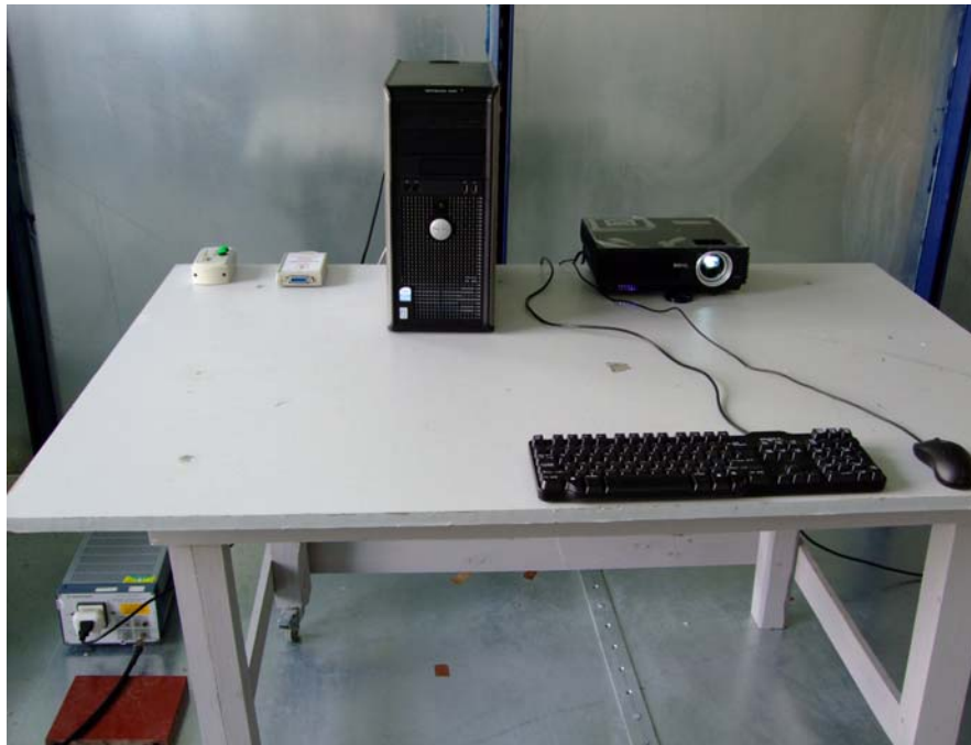
Conducted Emission Test Set-up - Front View
