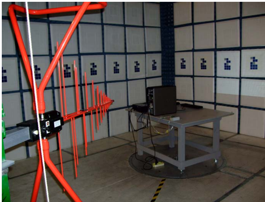
Radiated Emission Test Set-Up – Back View
