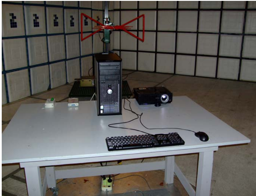
Radiated Emission Test Set-Up – Front View
