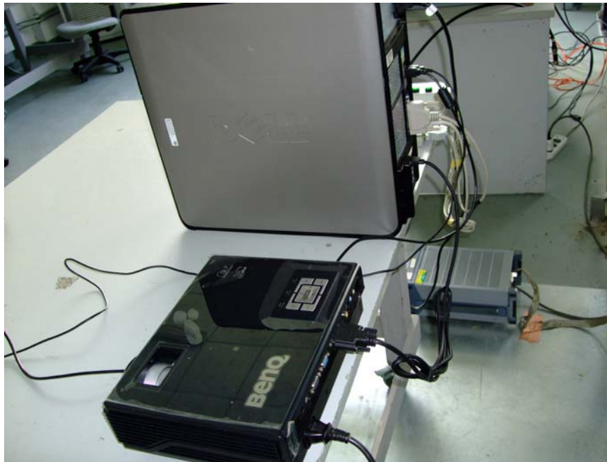
Conducted Emission Test Set-up - Side View
