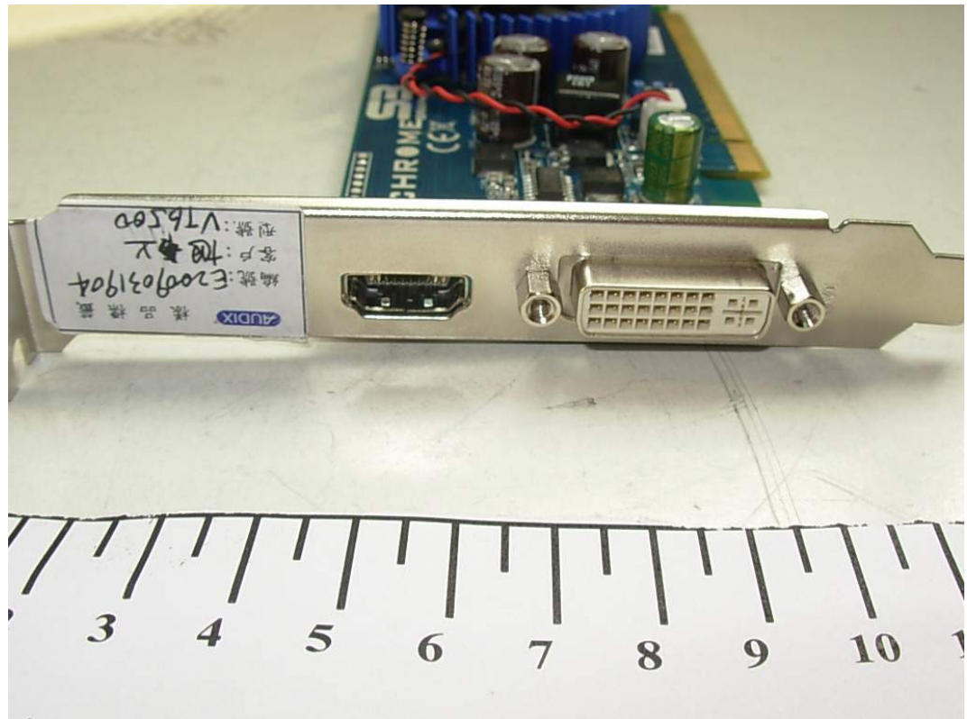
FIGURE 1 CHROME 430/440 GRAPHIC CARD (M/N: VT6500) GENERAL APPEARANCE (PORTS VIEW)
