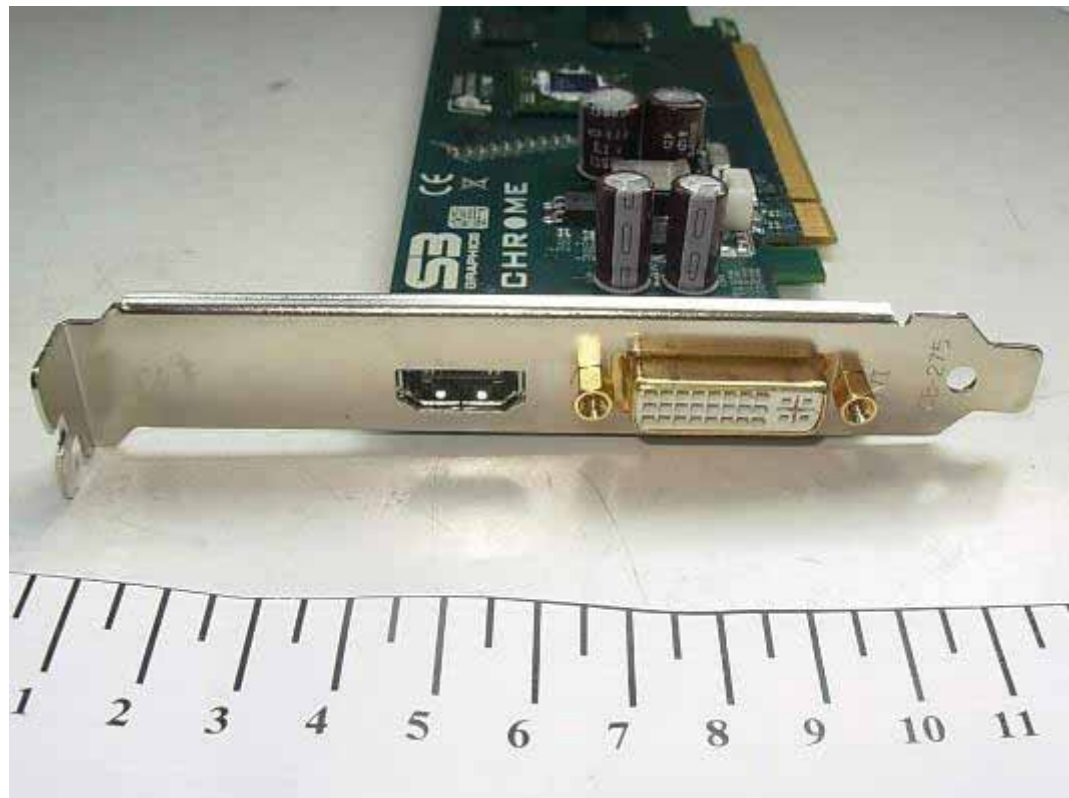
FIGURE 1 CHROME 530 GRAPHIC CARD (M/N: S3G003) GENERAL APPEARANCE (PORTS VIEW)
