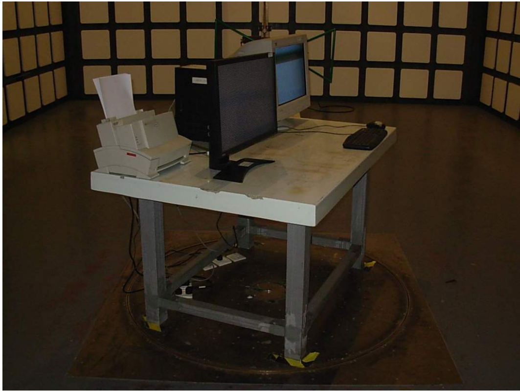
SETUP WITH MAXIMUM DETECTED EMISSION AT HORIZONTAL POLARIZATION (DVI + HDMI 2048*1536@60Hz)
