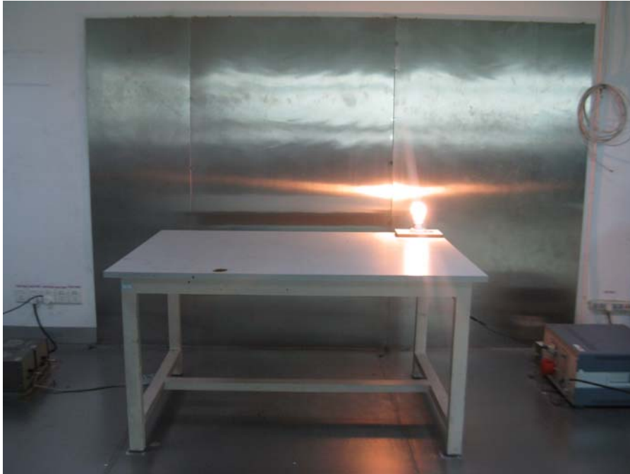
ELT-N818: Conducted Emissions - Side View
