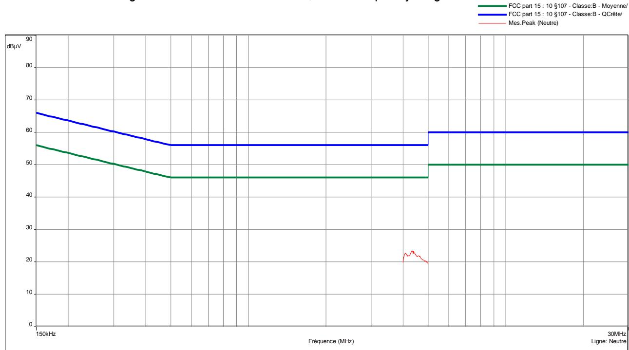
Curve N° 4: average measurement on the Line, for the frequency range: 4MHz to 5MHz
