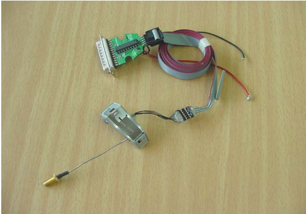
Conducted RF measurements _EUT with the TEST JIG used
