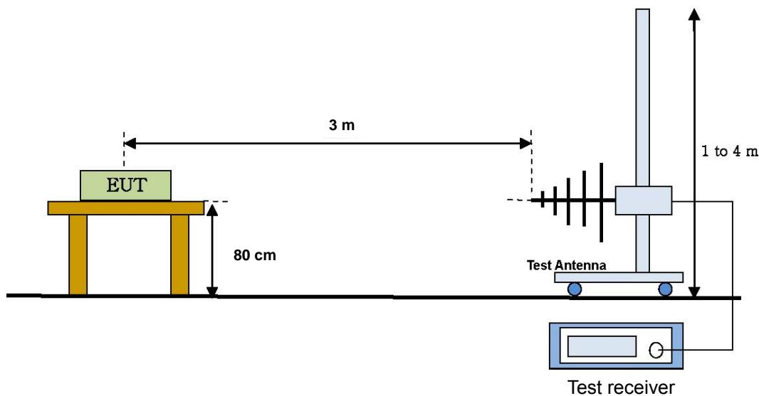
※ In case of above 1 GHz is using the Horn antenna instead of Broadband Antennal
