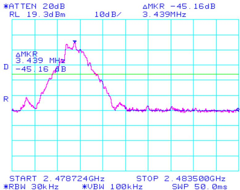
※ Above measured delta value is displayed at band edge point from lowest and highest frequency
