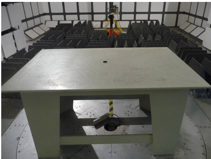
Radiated Emissions View (1-25 GHz)
