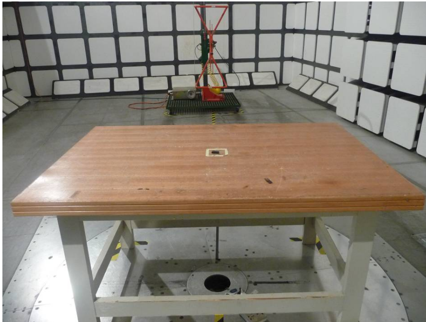
Radiated Emissions View (30-1000 MHz)
