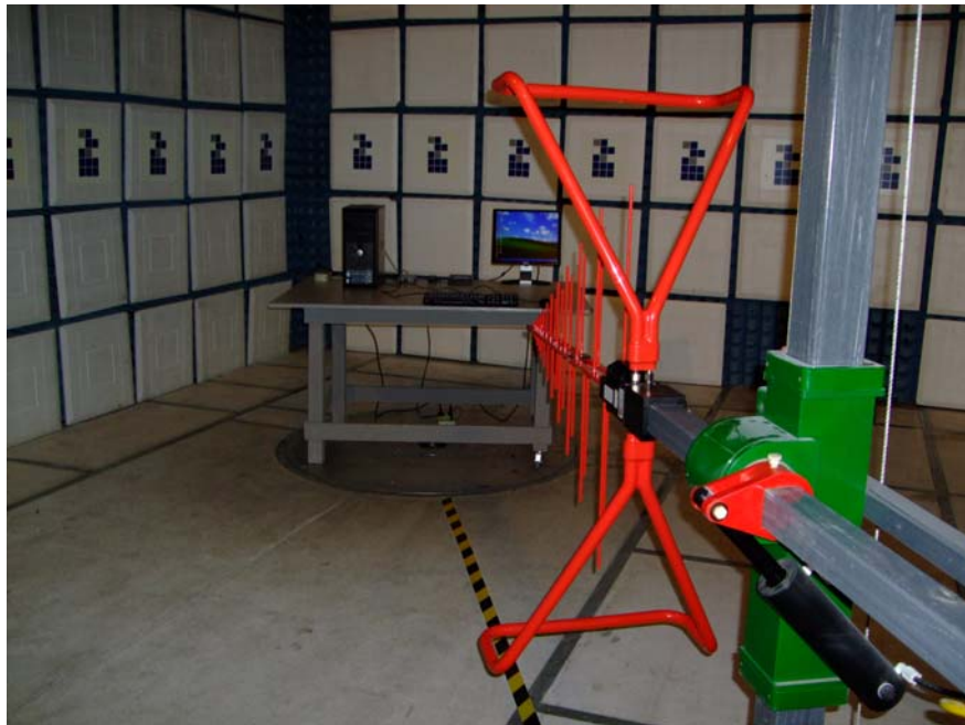
Radiated Emission Test Set-Up – Back View
