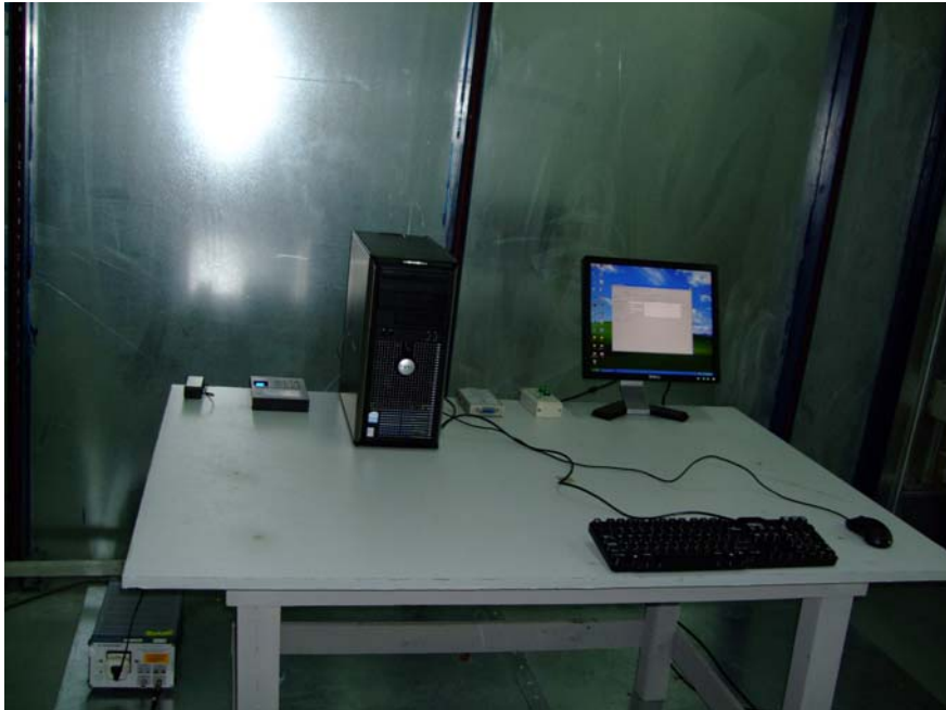
Conducted Emission Test Set-up - Front View
