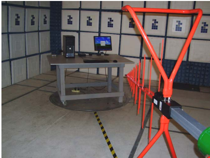
Radiated Emission Test Set-Up – Back View
