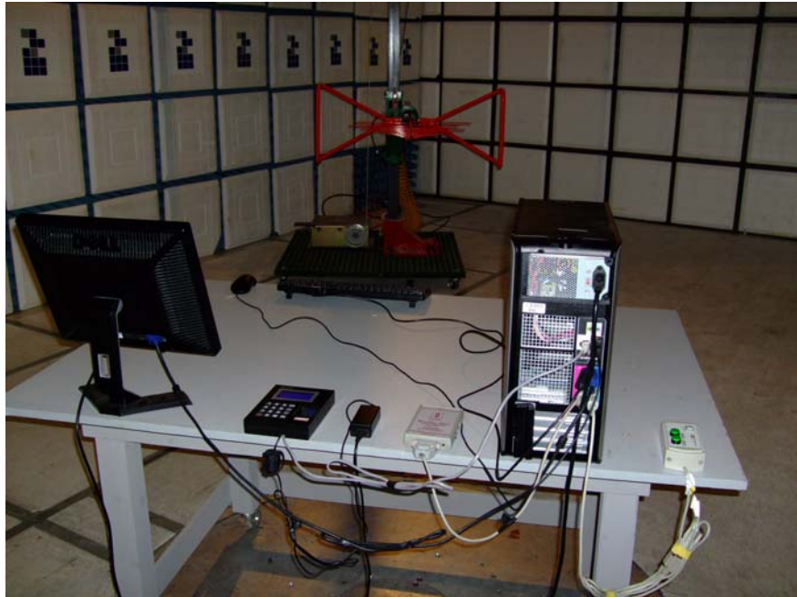
Radiated Emission Test Set-Up – Front View
