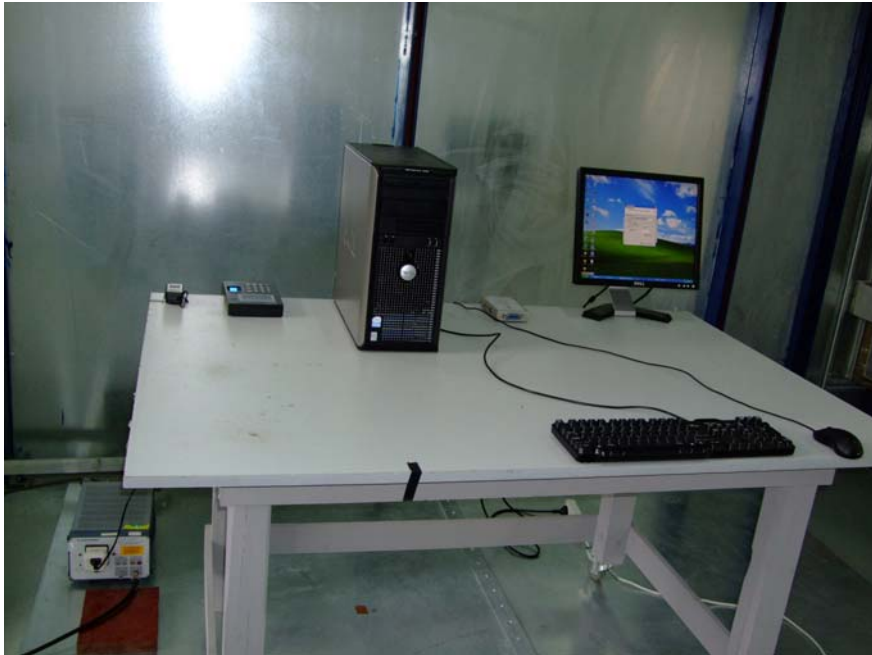
Conducted Emission Test Set-up - Front View
