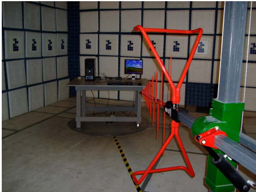
Radiated Emission Test Set-Up – Back View
