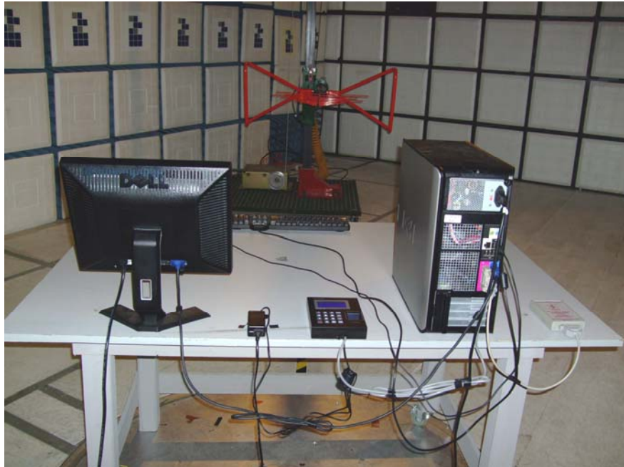
Radiated Emission Test Set-Up – Front View
