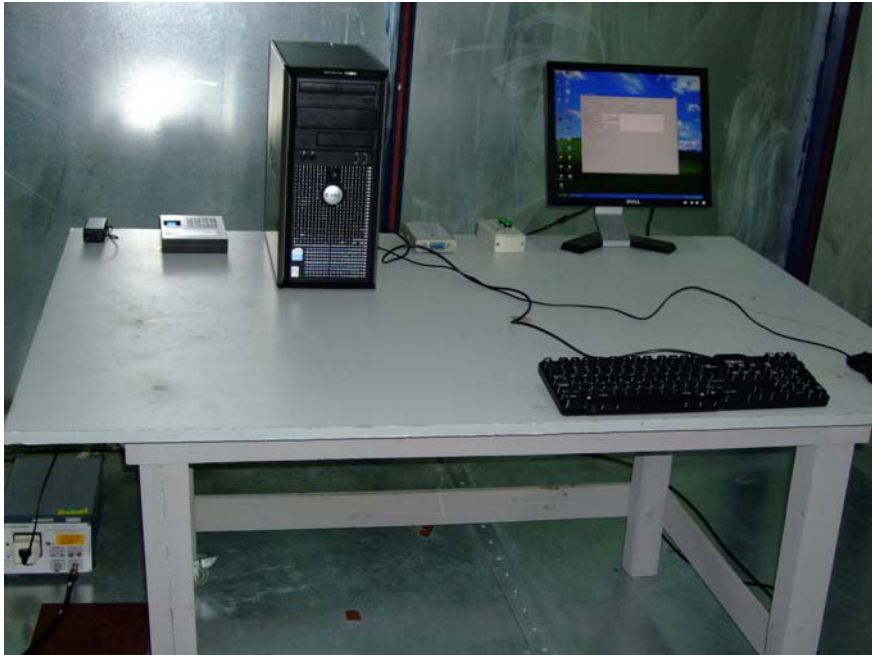
Conducted Emission Test Set-up - Front View
