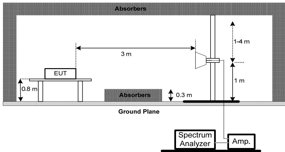
(C) For radiated emissions below 30MHz
